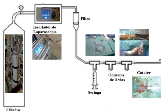
Figure 01: schematic diagram of the homemade delivery system
